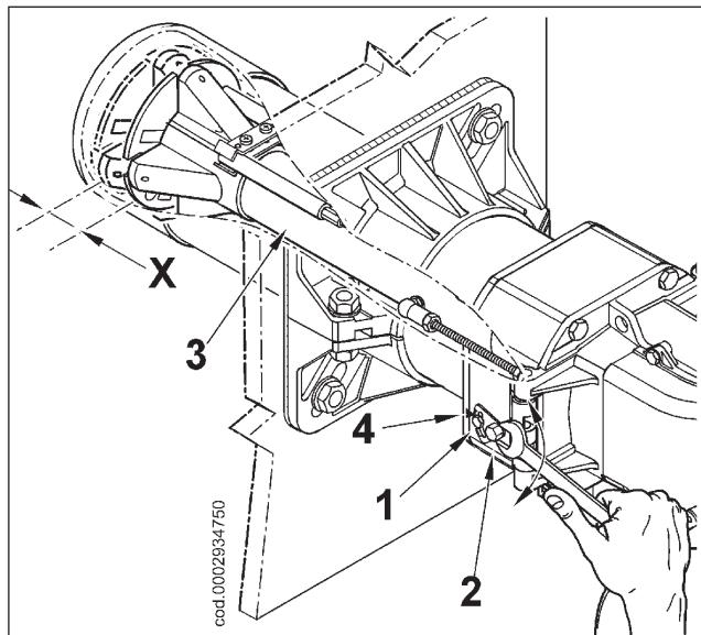
X= Combustion head-disk distance; adjust the distance X following the indications below:
