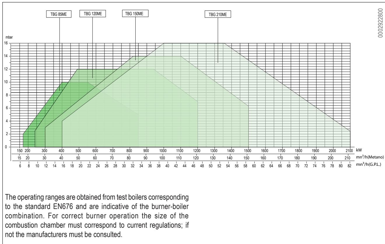
The operating ranges are obtained from test boilers corresponding to the standard EN676 and are indicative of the burner-boiler combination. For correct burner operation the size of the combustion chamber must correspond to current regulations; if not the manufacturers must be consulted.
